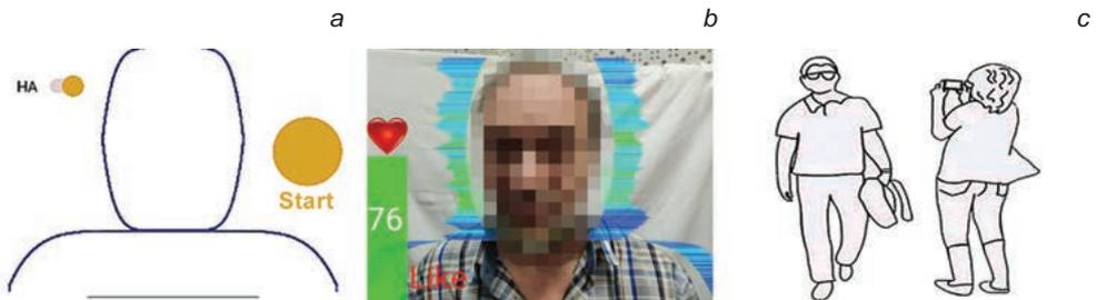
**Fig. 1.** The calculated contour separating the vibrations of the subject and the background in the frame (a), the result of the output of the correlation coefficient of the operator and subject microvibrations on the mobile phone screen after 10 seconds of testing (b), and a schematic representation of the compatibility testing of the operator and subject (c)
